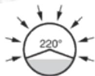
LP locally perforated pipes
