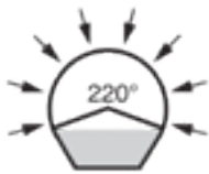
LP locally perforated pipes
